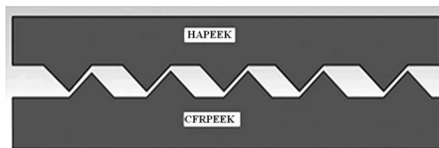
Figure 1. Shape of energy directors at the interface.
